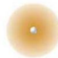
FIGURE 1.1 The exact position of electrons cannot be known. They are somewhere in a three-dimensional electron cloud around the nucleus.
